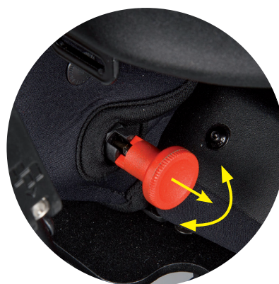
Twist lock - Open (pull and turn 90° until it gets into a small groove that keeps it in the open position.)
